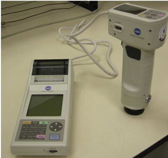
FIGURE 8.1 A Minolta colorimeter (Minolta Camera Co. Ltd, Osaka, Japan, Fig. 8.1) used for quantitative food and beverage colour measurements.
