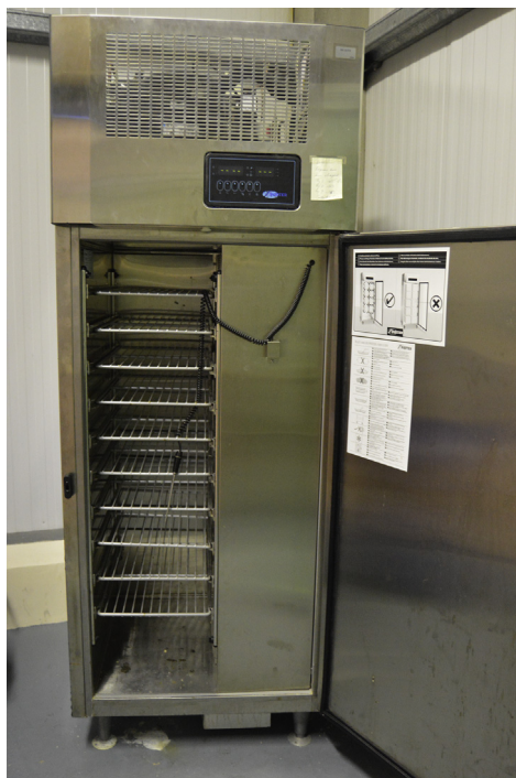
FIGURE 6.2 Displays a Foster F35 Blast Freezer. The high-powered refrigeration system blasts cold air laterally over the product at high speed, extracting heat at an optimum rate, while maintaining food quality. Once the cycle is complete, the equipment switches into ‘hold mode’ to keep the food at the required temperature.
