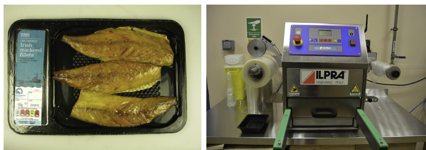
FIGURE 7.2 Vacuum skin packed mackerel fillets and an ILPRA (Vigevano, Italy) vacuum skin packaging machine.
