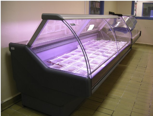
FIGURE 6.3 Retail refrigerated display cabinet used for shelf life assessment (O'Sullivan, 2011b, 2016).
