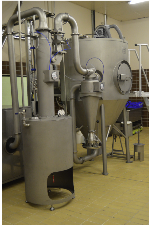
FIGURE 12.1 GEA-Niro Production Minor spray dryer. Presented is a single stage drying unit (main chamber and cyclone collection) fed by either rotary disc or nozzle. Drying conditions range from 170 to 190°C inlet and 70–90°C outlet with full digital control. Drying capacity is ~15 L/h (30% TS solution) to dry 5 kg powder.
