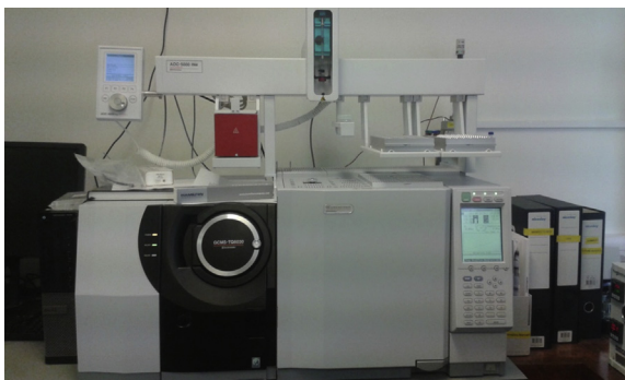
FIGURE 8.3 Shimadzu 8030 TQMS (Triple Quadrupole Mass Spectrometer) with Combipal autosampler (CTC analytics, Basel, Switzerland).
