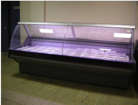
FIGURE 11.4 Retail display cabinet used to simulate commercial retail display conditions. It is important when using such equipment that the light intensity (LUX) is recorded as well as operating temperature fluctuations using a data logger.
