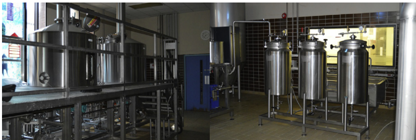
FIGURE 13.3 The picture on the left depicts a 1000-L pilot scale brewery. On the right is a 50-L brew house. This small 50-L brew house consists of a mashing, lauter and wort boiling kettle. The whirlpool, cooler and the three 50-L fermenters ensure a standardised operation and performance in small half technical scale.
