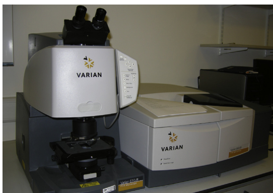
FIGURE 8.4 Fourier transform infrared (FTIR) spectroscopy. Presented is an Agilent 670IR with 620 microscope.
