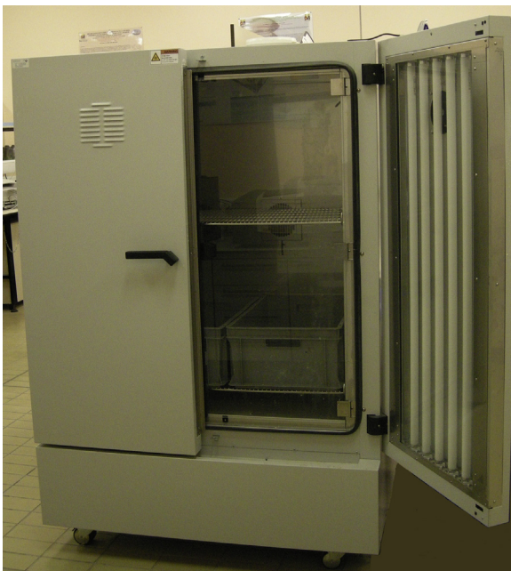
FIGURE 6.1 Displays a Binder (BINDER GmbH, Tuttlingen, Germany) climatic cabinet (KBF 720) which are used for accelerated storage testing. Temperature, humidity and light parameters can be controlled with ranges from -10 to 100^{\circ}\text{C} without humidity and lighting, 10 – 90^{\circ}\text{C} with humidity and 20 – 90^{\circ}\text{C} with humidity and lighting. Photo stability testing can be undertaken with the doors incorporating Lux 4000 lighting. In the system presented, a remote data recording system has been incorporated. These wireless recorders communicate by radio frequency with the server PC at defined regular intervals and record many different parameters such as temperature and humidity in this case, but can also record additional measurements, depending on the application such as hygrometry measurements or pressure if required (O’Sullivan, 2011b, 2016).
